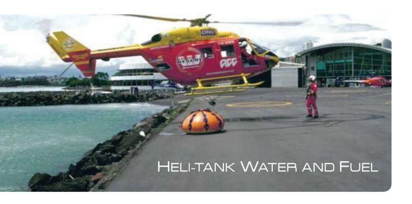
The **Heli-Tank** is a collapsible tank designed primarily to be slung beneath Helicopters to fly water or fuel rapidly to remote or inaccessible locations. The specifically designed pod shape of the tank enables stable flight when full or partially full, enabling partial offloading en route.
