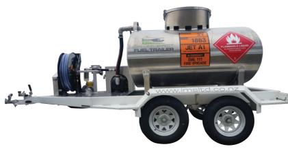
1875 Litres capacity, incorporating a full filtration system with flow metering unit.
