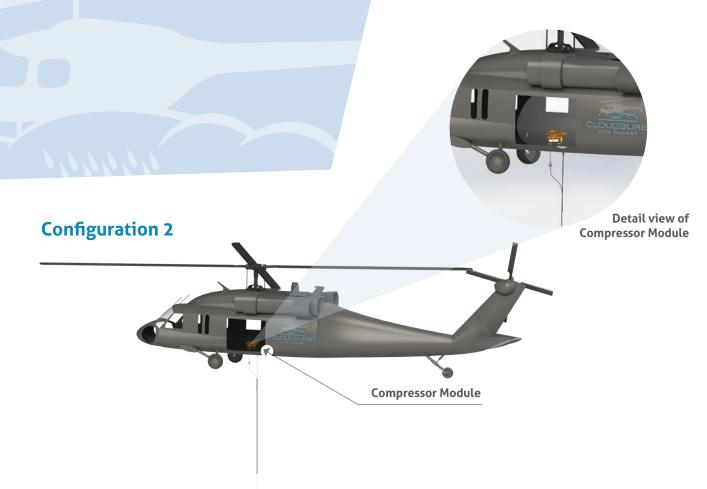
**Configuration 2** offers a **Compressor Module** that sits inside the aircraft and provides compressed air supply to the Cloudburst Bucket. This module can have a corded remote control to operate the bucket by crew members. It also can be coupled with our **Power Control Module**, which provides an auxiliary power supply to operate the entire system.
