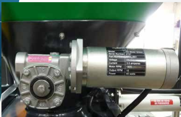
Agitator drive system. Rotates when Slide Valve is open.
