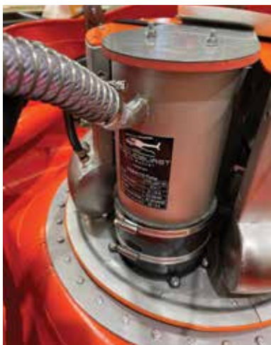
Monsoon Valve Mounted DC Pump (single)
