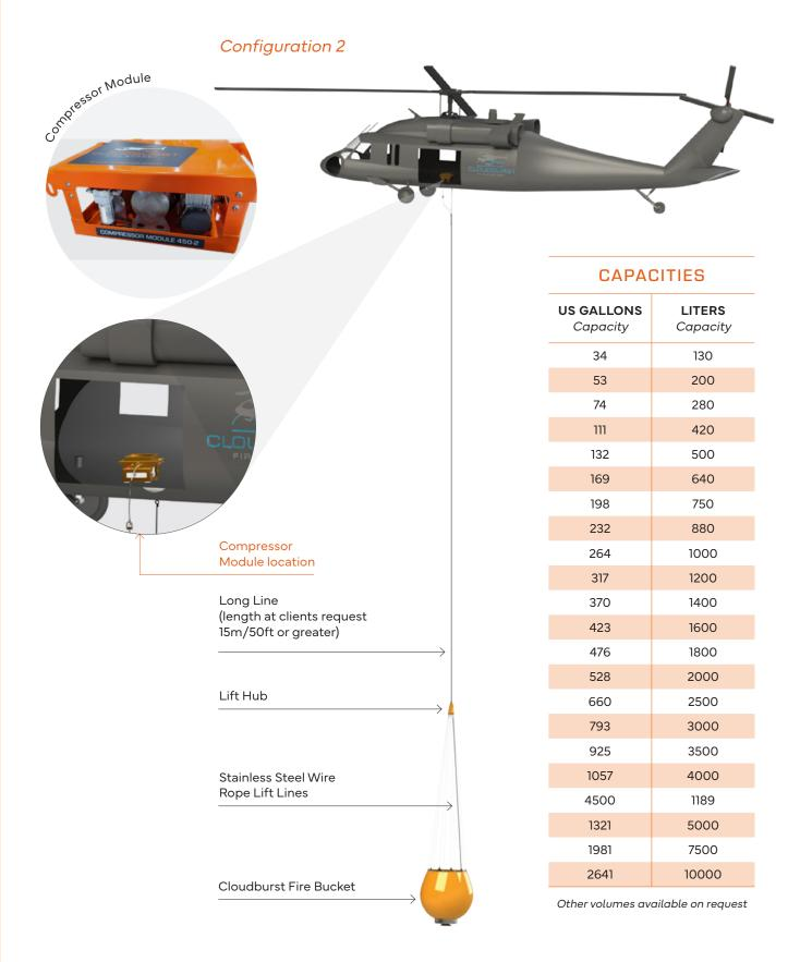
Configuration 2 requires a Compressor Module, located inside the aircraft that provides compressed air supply to the Cloudburst Fire Bucket. This module has a corded remote control for crew members to operate the Cloudburst Fire Bucket. It also can be coupled with our Power Control Module, which provides an auxiliary power supply to operate the entire system. Many combinations can be used to accommodate the needs required to operate your Cloudburst Fire Bucket system.
